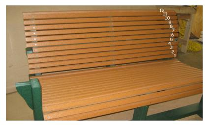
Notice that the seat slats are numbered on the underside of each slat - they will be attached to the frame later - for now, just start the screws.
