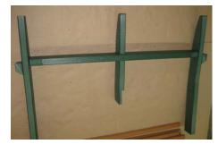
Step 1&2:: Assemble the front and rear leg sections as shown above.
